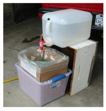
1) **FILLING FROM PREPARED KEGS.** NEVER MOVE THE ACID FILLED CONTAINERS WITHOUT SECURELY INSTALLING FULL LIDS AND AIR VENT PLUG. DO NOT MOVE CONTAINERS WITH TAPS.
