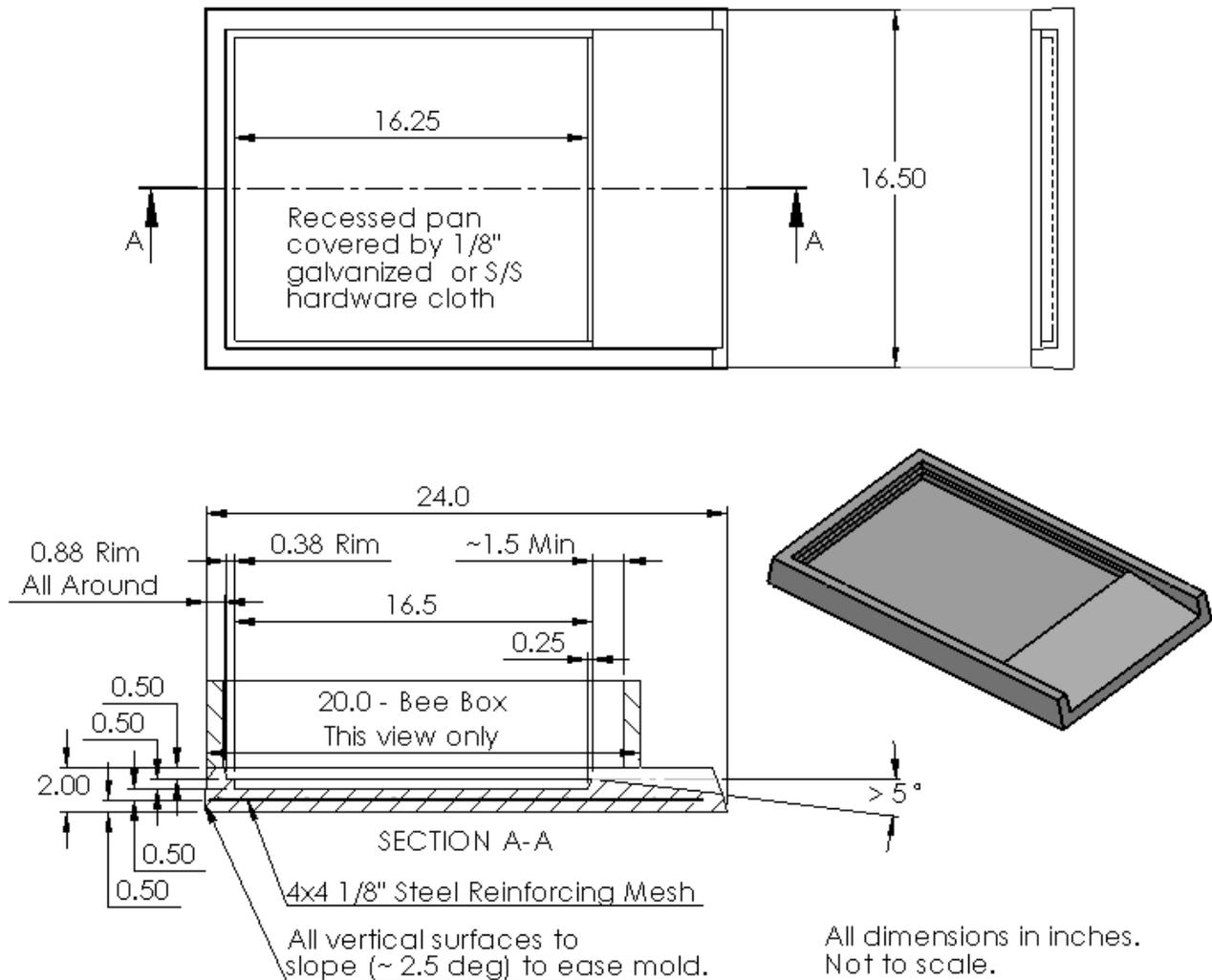
**MATERIAL** for tropical stationary beekeeping: Fine concrete or fired clay as used for pottery.
