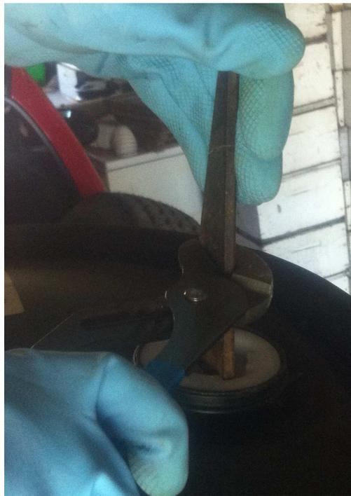
You need a piece of steel to fit between the wrench opening of plug and large channel lock pliers. Turn to the right and
